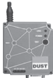
Fig. 29.7.4: Dust Networks Evaluation Mote
